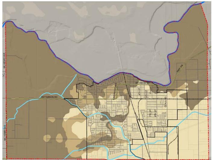
Figure 3–7 Depth to Hardpan Condition
