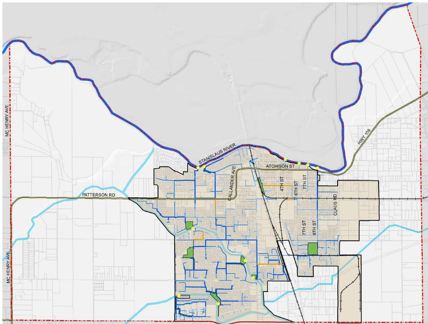
Figure 3–10 Existing Storm Drain System Infrastructure
