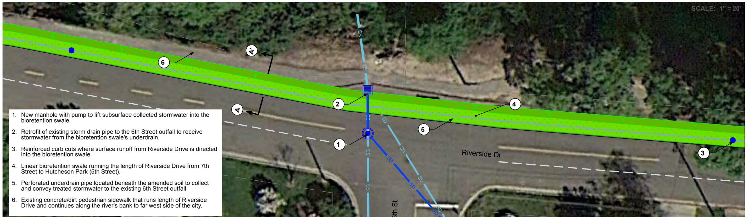
1. New manhole with pump to lift subsurface collected stormwater into the bioretention swale.
