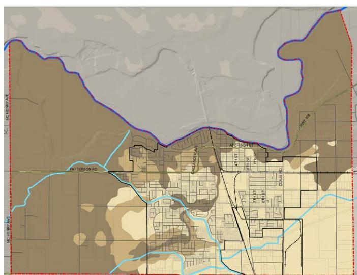
Figure 3–7 Depth to Hardpan Condition
