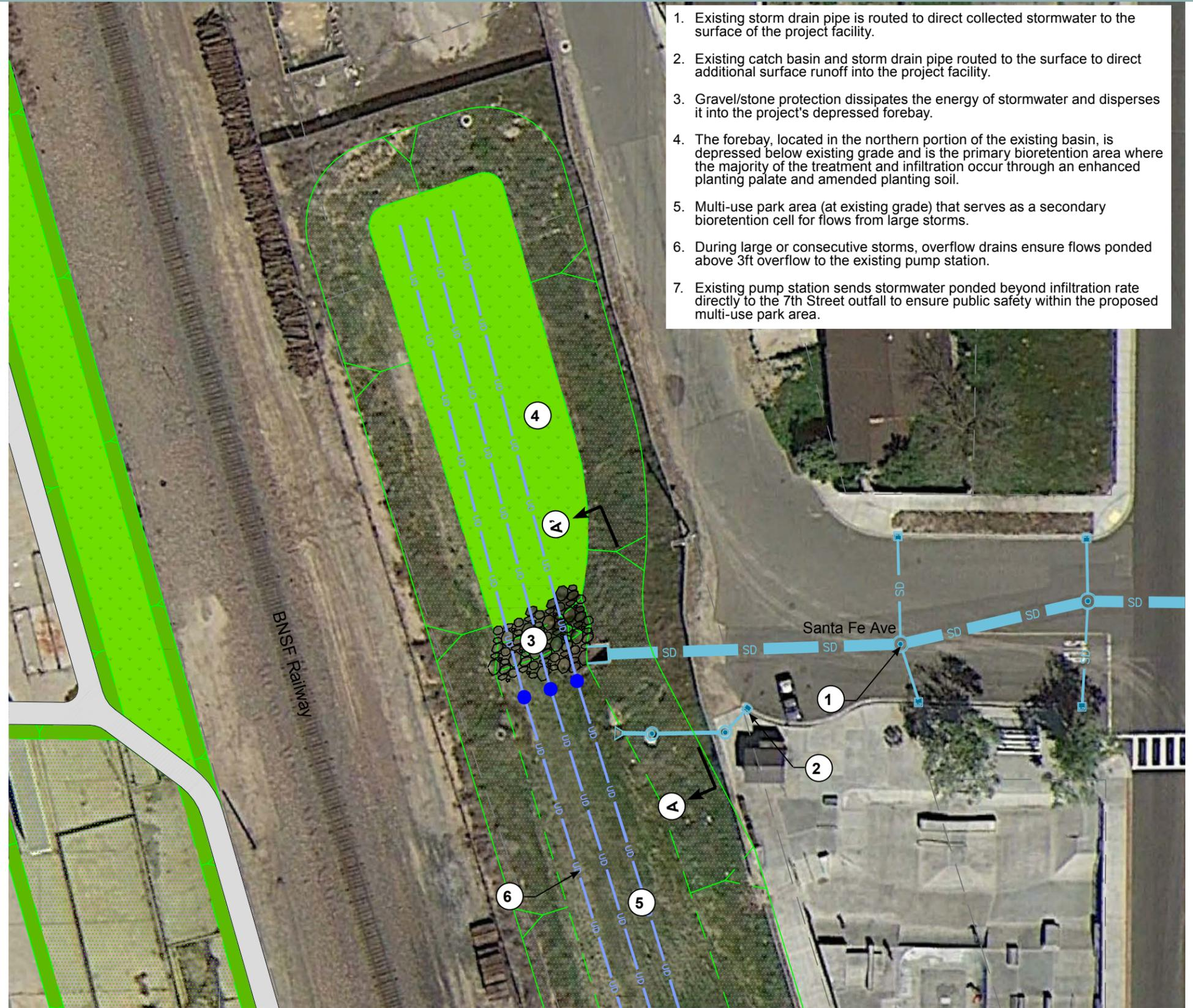
1. Existing storm drain pipe is routed to direct collected stormwater to the surface of the project facility.
