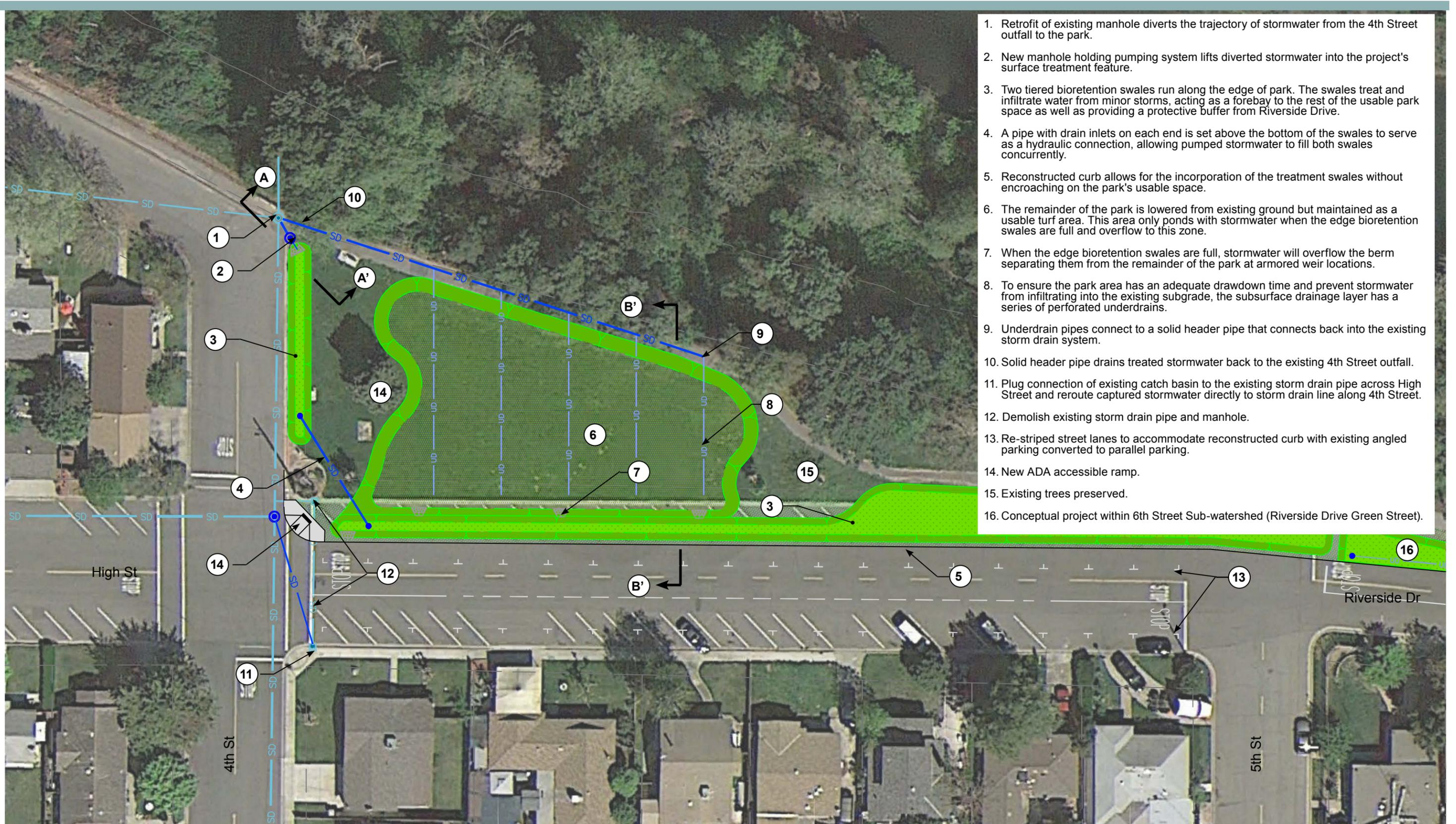
1. Retrofit of existing manhole diverts the trajectory of stormwater from the 4th Street outfall to the park.
