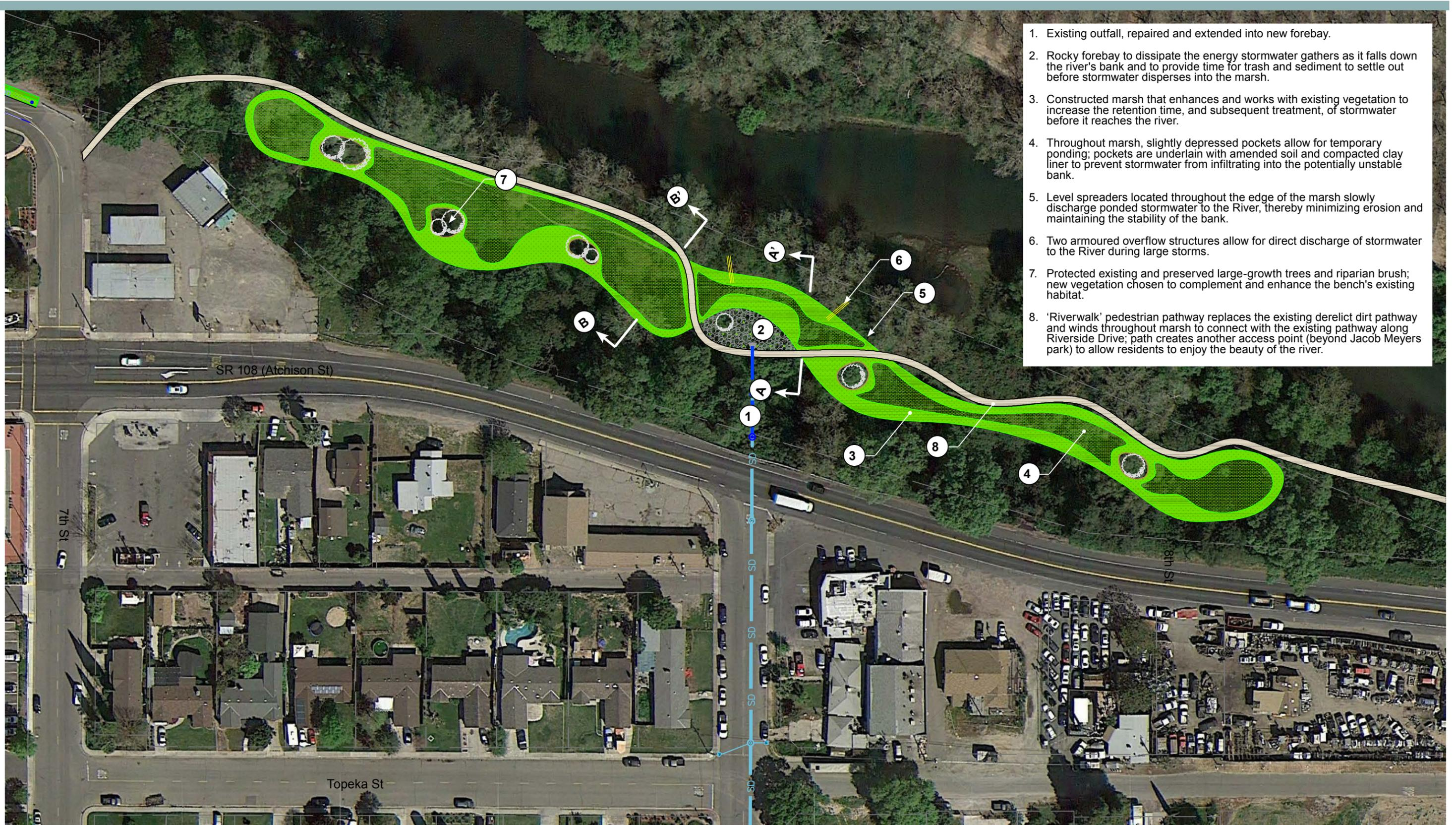
1. Existing outfall, repaired and extended into new forebay.
