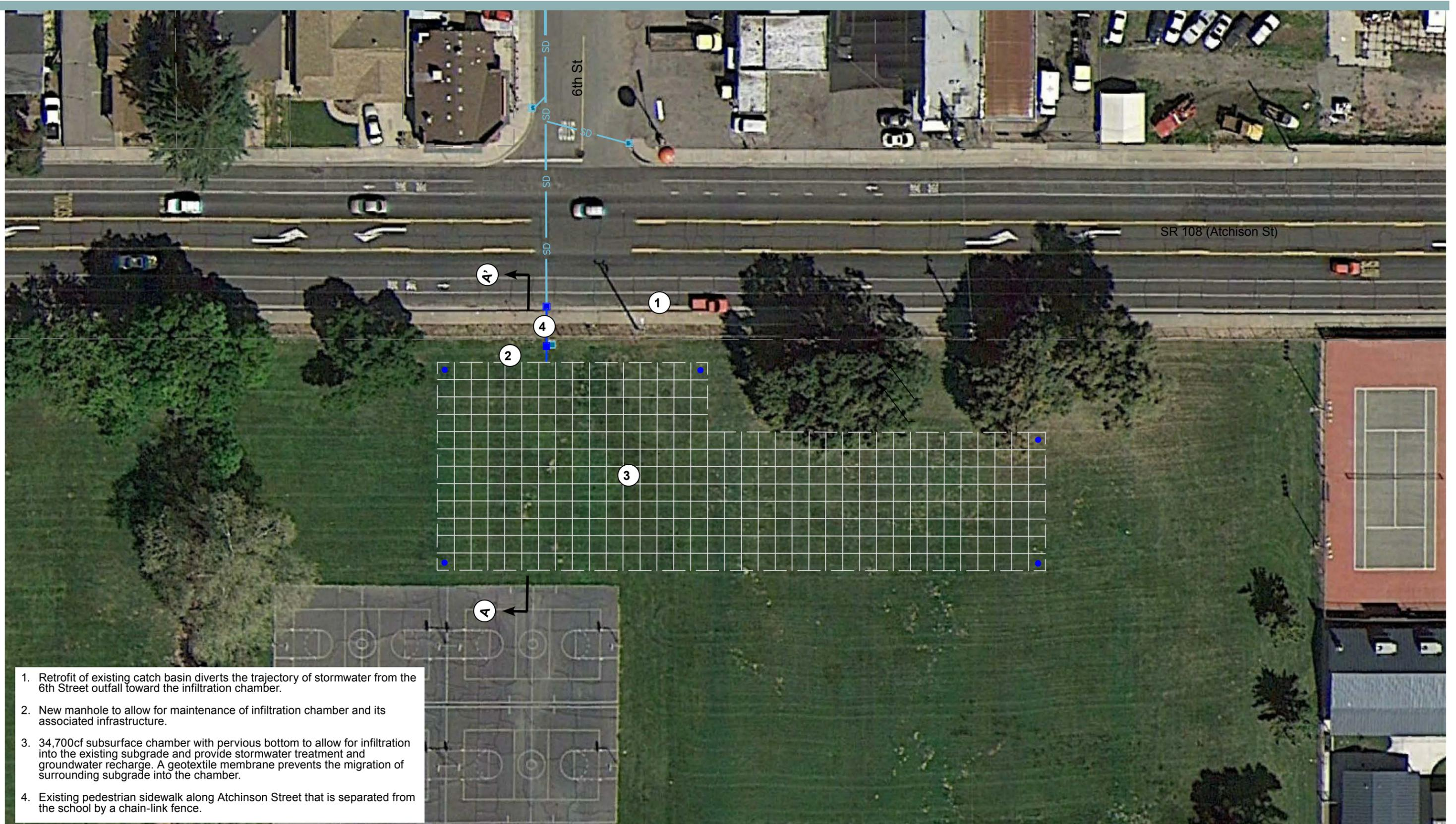
1. Retrofit of existing catch basin diverts the trajectory of stormwater from the 6th Street outfall toward the infiltration chamber.
