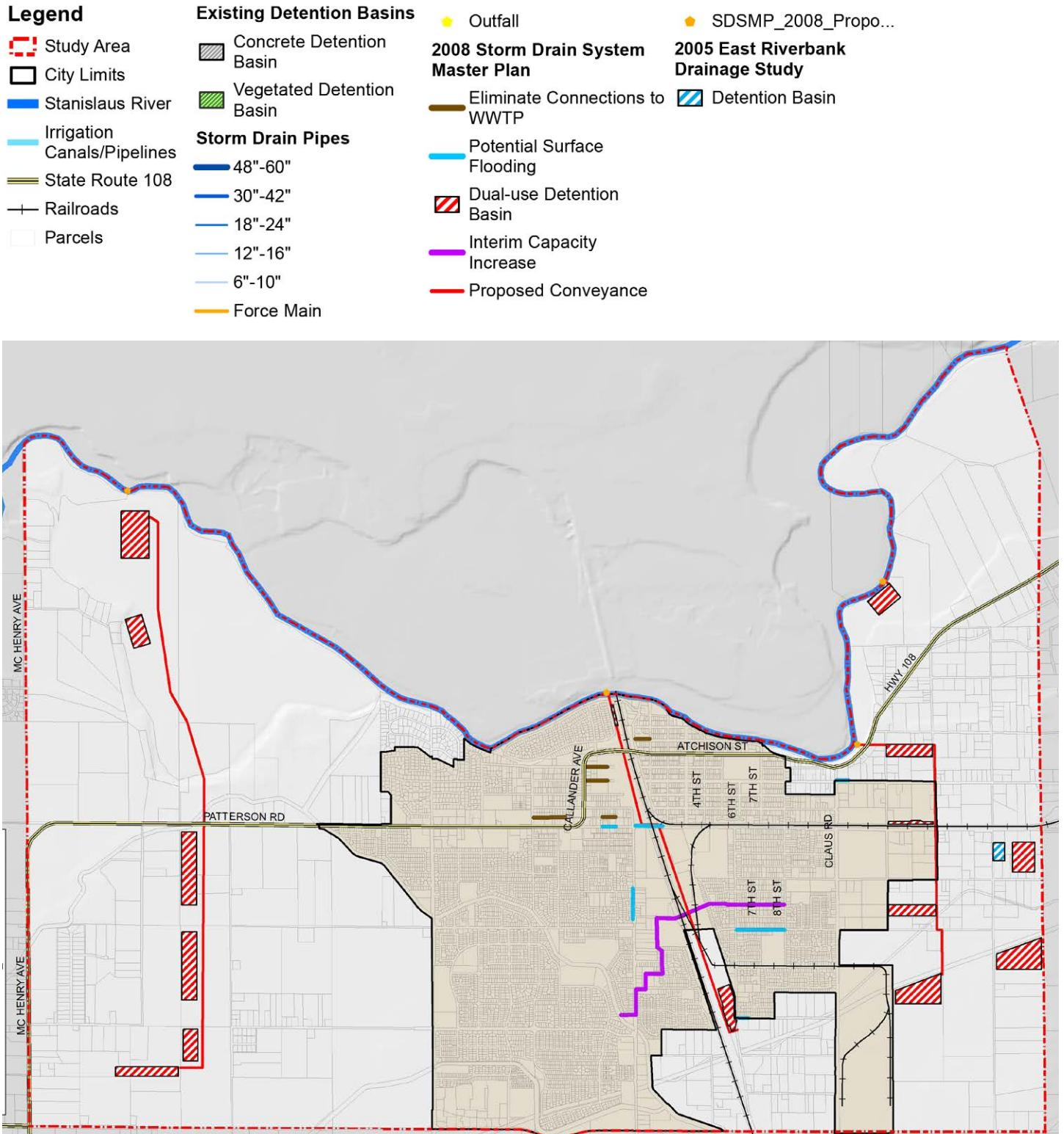
Figure 3–11 Storm Drain System Infrastructure Already Proposed
