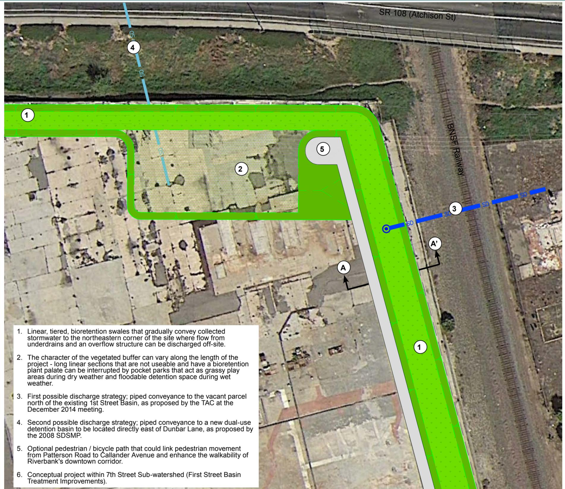
1. Linear, tiered, bioretention swales that gradually convey collected stormwater to the northeastern corner of the site where flow from underdrains and an overflow structure can be discharged off-site.
