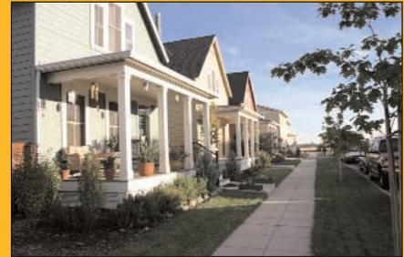
A wider sidewalk, with a planting strip next to it, provides a buffer between moving vehicles and pedestrians.
