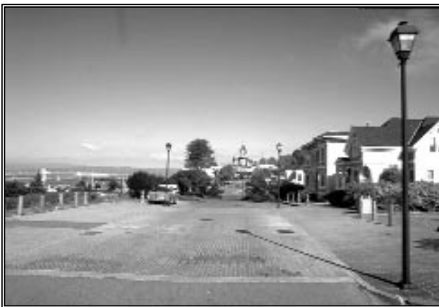
This Eureka, California, street has a raised intersection, which uses colored, textured pavers to make the street more attractive.
