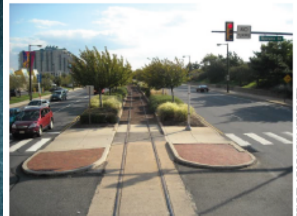
Figure 2-4: This arterial street emphasizes multiple transit options. The center median has a street car line, bike lanes flank both sides of the street, buses share travel lanes with autos, and pedestrians can safely cross street intersections.
